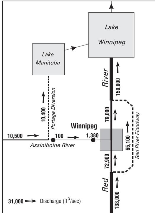
**Figure 5:** Routing of flow on May 4, 1997.
